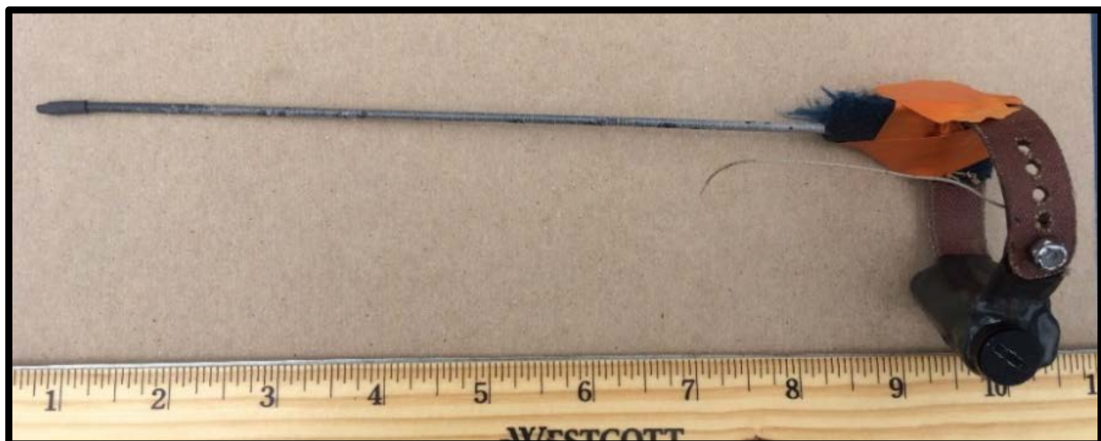
Figure 2. ATS G10 UltraLITE collar used to study martens in northern Wisconsin. Total collar mass (including VHF and GPS components) was 27 g.
