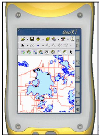
**Figure 3.** GPS receiver running ArcPad.
